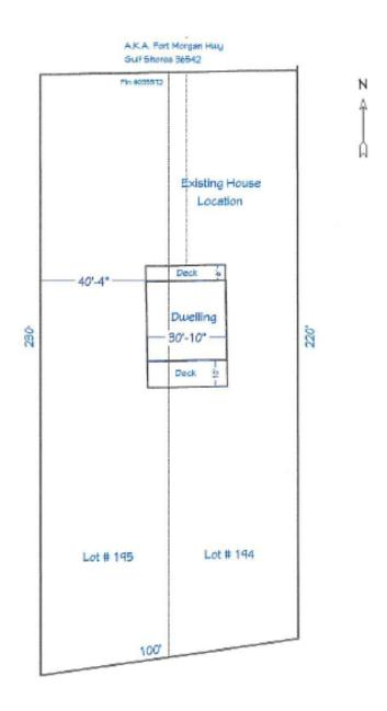
This drawing of existing house location does not match aerial photography which shows an addition on lot 195 in 2017. Contacted the property owner for accurate information.
